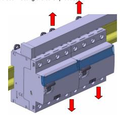
Put the latch clips in the unlocking position
